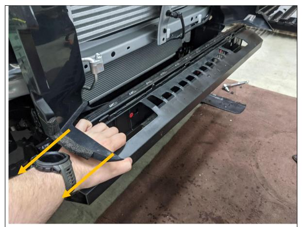
25. Remove the plastic cover from the impact beam by strongly pulling in the direction shown to release it from the clips
