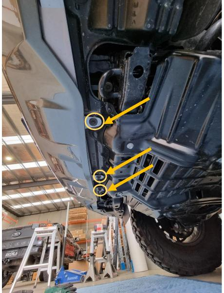
11. Remove the 3x Factory Screws securing bottom center section of bumper to inner wheel arch liner. Use 10mm socket / spanner.
