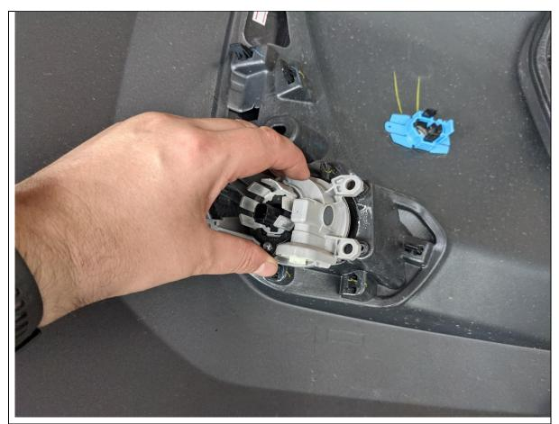
50. Remove the 3x Screws securing the fog lights to the bumper, then remove the fog light from the bumper
