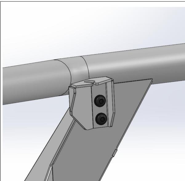
121. For Toro bars, if fitting antenna fit the antenna brackets to the captive nuts in the uprights using supplied M8x20 Button head bolts, and flat washers
