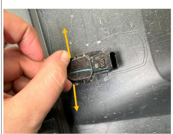
51. Remove parking sensors from housings, by prying apart the locking tabs, whilst pushing sensor from front side of bumper.
