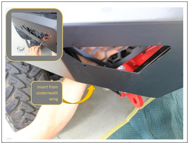
106. Fit light mesh panels to the bar. Position the panel from underneath the bar and align with the mounting holes in the wing. Secure with 4x M6x16mm Button head bolts and M6 Flange Nuts
