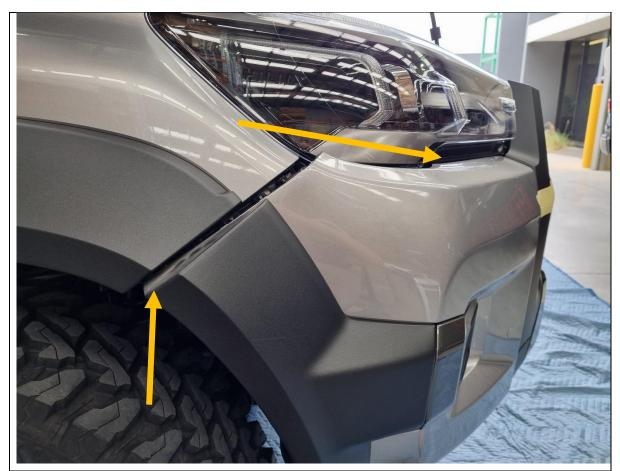
13. Remove the bumper. Start by pulling from the outside where the bumper meets the wheel arch and work towards the center from both sides.
