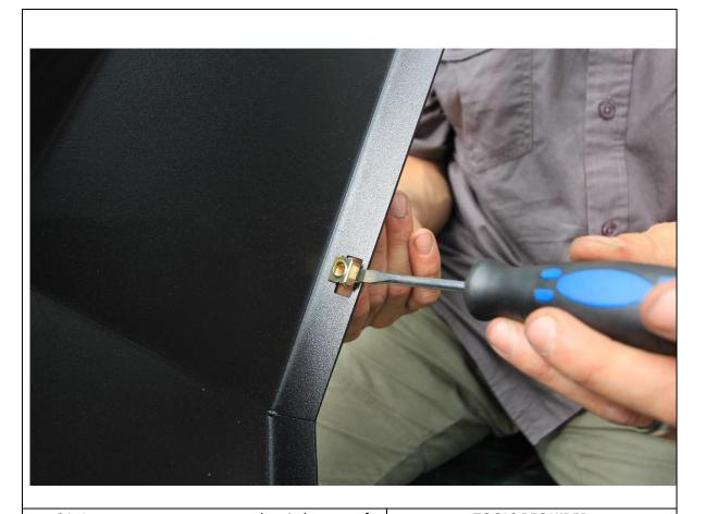
84. Insert cage nuts to square slots in bottom of wings. Seat cage nut against one edge of slot then push other edge in with flat bladed screwdriver.
