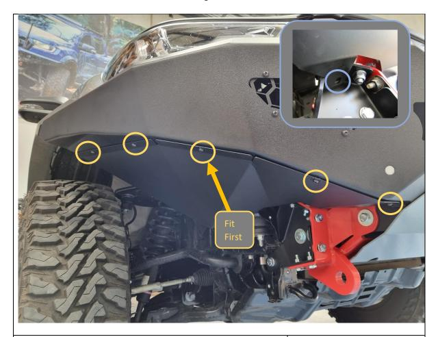
114. Fit side under panels to bar and secure with 4x M6x16 Button head bolts and M6 Flat washers, into M6 cage nuts fitted earlier.
