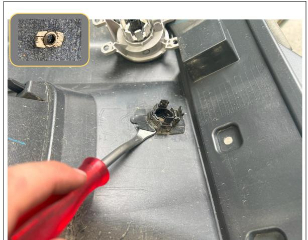
52. Carefully pry the sensor housings away from the back of the bumper, using a trim tool or similar.
