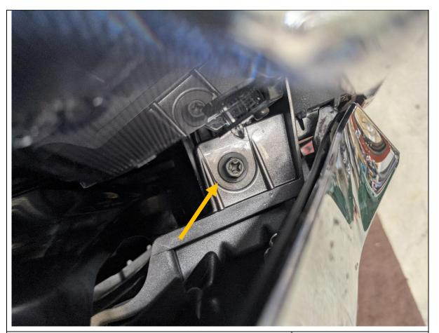
12. Remove the 2x 10mm Head/Phillips screws securing the bumper to crossmember.
